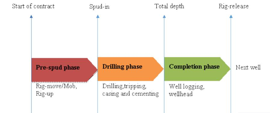
FIGURE 1: Summary of the phases of geothermal drilling
