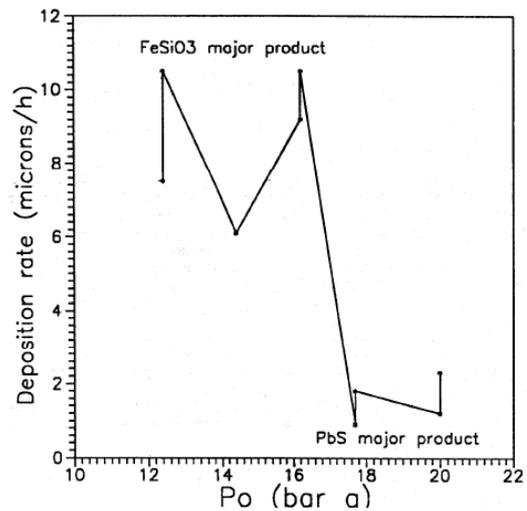
**FIGURE 4 : Thickness of scales on coupons at different pressures (Ármannsson and Hardardóttir, 2010).**
