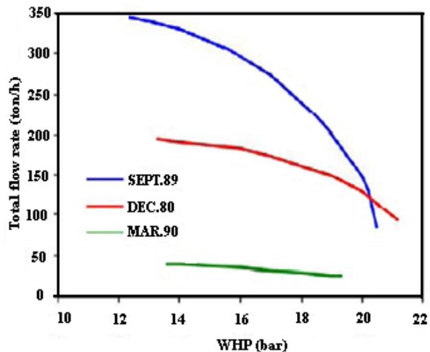
**FIGURE 6: Output characteristic curves for different test well Asal 3 (Jalludin, 2009).**
