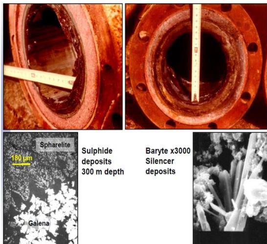
**FIGURE 5: Scale deposits in 6 inch production Liner Asal 1 geothermal well**
