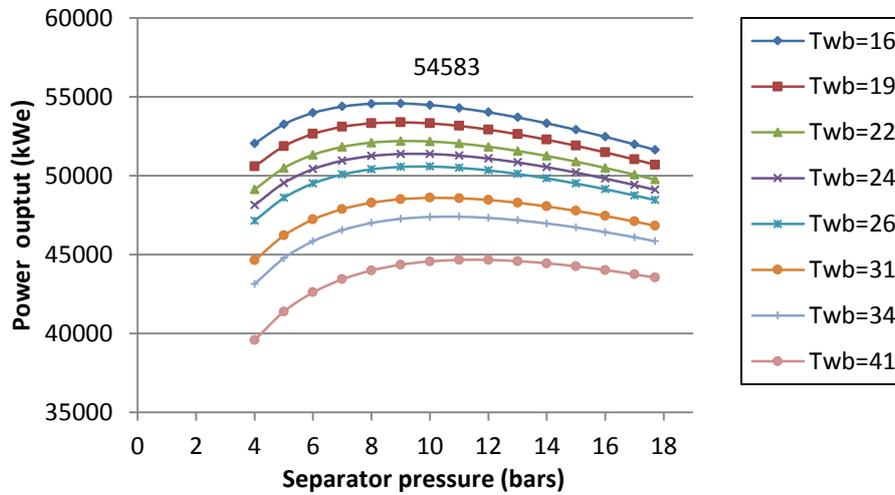
FIGURE 8: Separator pressure Vs Power output
