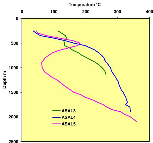
FIGURE 3: Temperatures profiles of wells A3, A4 and A5 (Jalludin, 2009).
