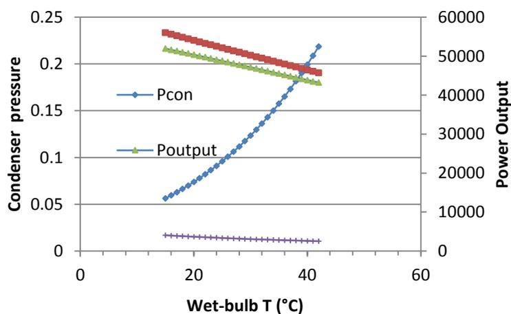
FIGURE 9: Wet-bulb temperature versus Poutput and condenser pressure
