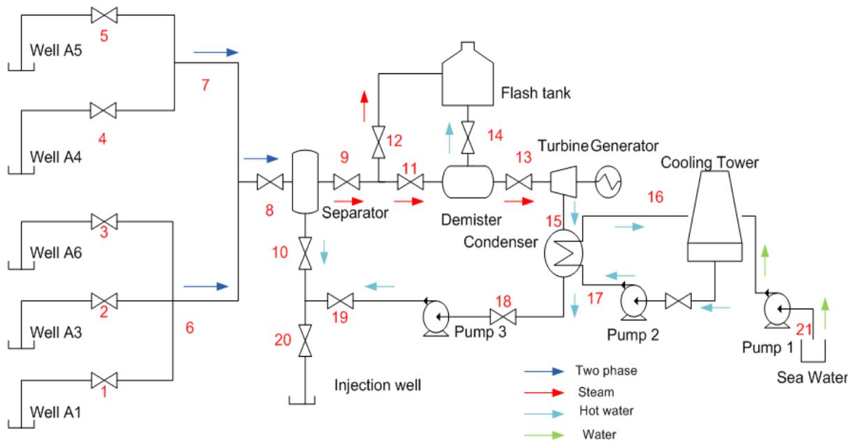
**FIGURE 7: Flow diagram of Asal geothermal power plant**
