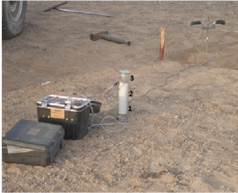
Figure 3: Using the RAD7 machine radon measurement is being taken in one of the stations.
