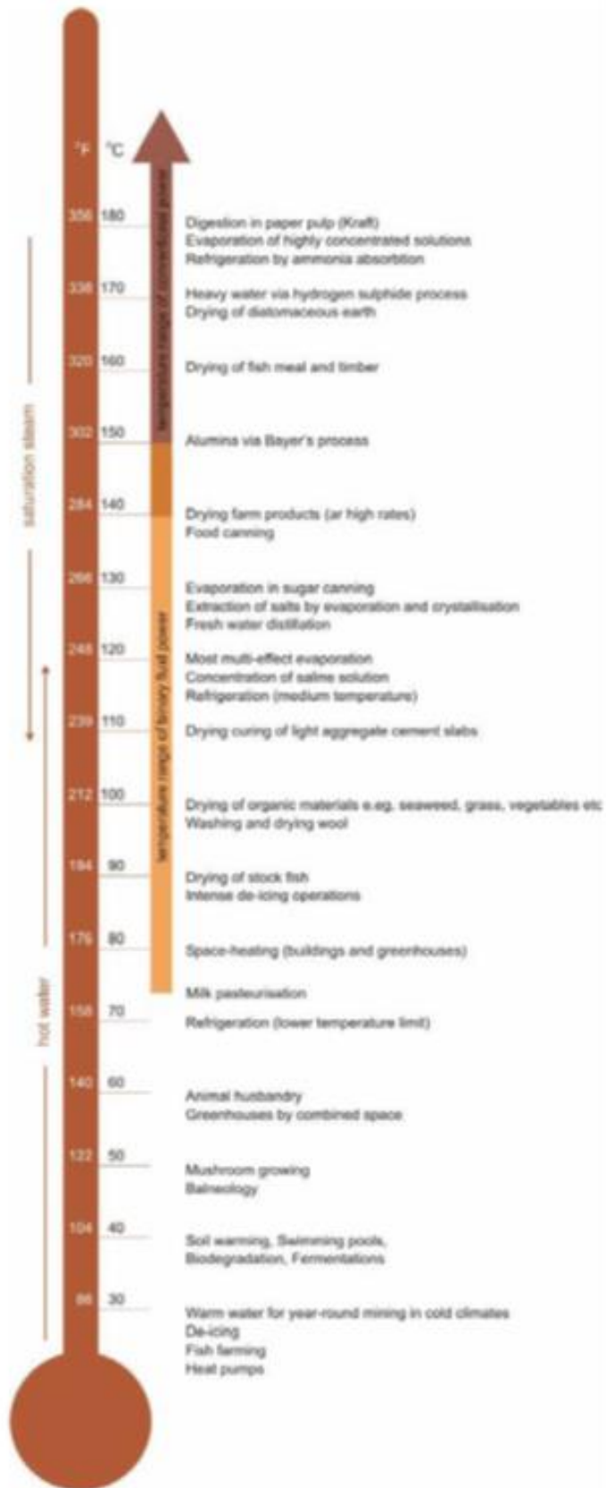
Figure 2: Lindal diagram showing utilization of geothermal energy depending on temperatures (Lindal, 1973)
