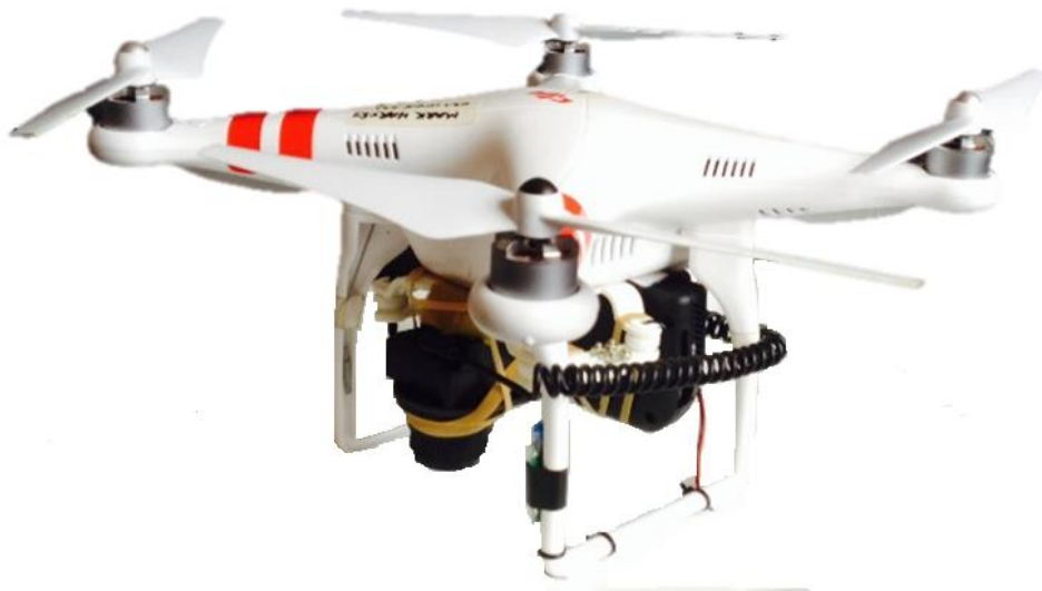
Figure 1: DJI Phantom 2 Vision Plus quadcopter modified with ICI thermal camera and UAV module
